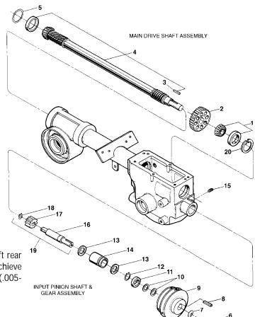
NOTE 1–Shim between drive shaft rear bearing and rear bearing cap to achieve 5-to-10 thousandths of an inch (.005-.010) end play on drive shaft.
